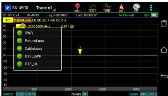
Figure 10 Selecting Cable Loss Measurement
