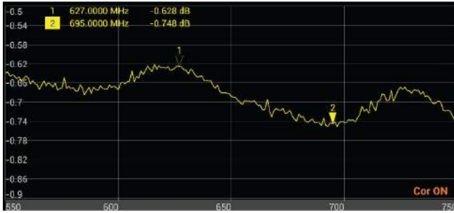
Figure 11 Interpreting Cable Loss Measurement
