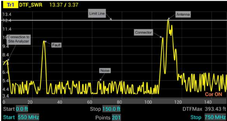
Figure 13 Interpreting Fault Location Measurement
