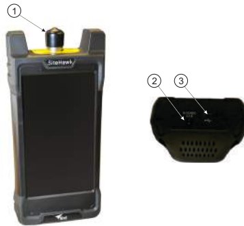
Figure 1 SK-4500 Connectors and Ports
