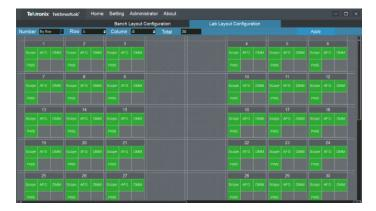
Instructors can easily monitor the status of all instruments during the experiment: Green signifies that the instrument is working, gray signifies no connection, and red signifies an error. An instructor can check on or help a specific bench by clicking the corresponding bench icon.
