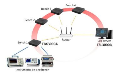
On the lab server, the TSL3000B communicates with the TBX3000A on each bench. The TSL3000B gives instructors centralized control of large fleets of instruments and gives students the ability to retrieve test results. and edit test reports online.
