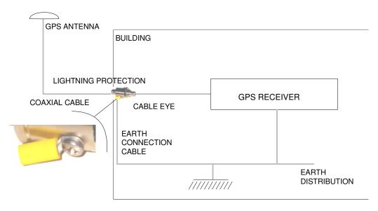
The lightning protection ground connection must have a very low impedance value. Use a section greater than 3mm2 and the shortest possible length of cable between the protection and the building ground connection.
