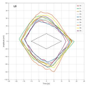
The major benefit of the Margin Tester is the speed at which a user can generate these eye diagrams. Since the eyes are shown to the user in real-time, it only takes seconds before results are displayed. This speed leads to dramatically reduced time to insights into DUT link health. With time to market pressures rising for engineers, Margin Tester steps up to provide insights to design and validation teams faster than ever before.
